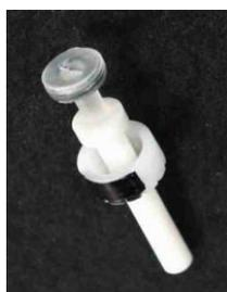
Zirconium Rotors (gHX compatible)
